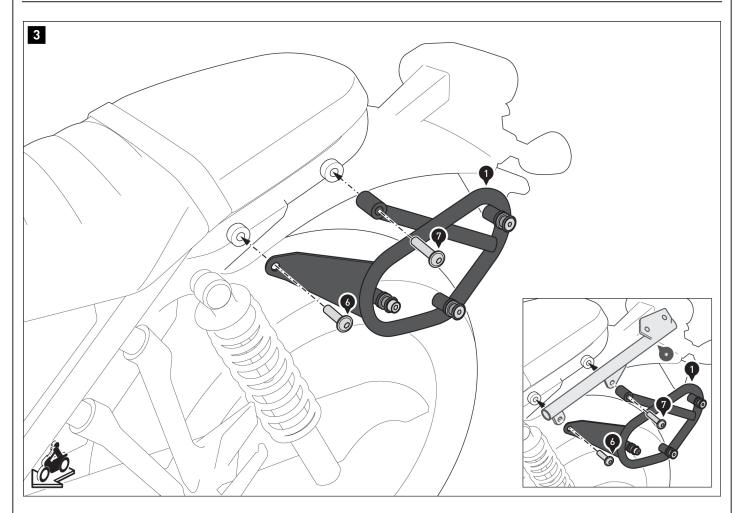
$\triangle$  **NOTE:** If you are installing the side carrier (1) with the SW-MOTECH rack (\*) at the same time, screw the parts together as shown in the detail drawing.
