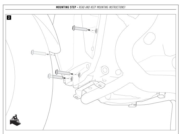
Remove the four original screws shown from the vehicle.
