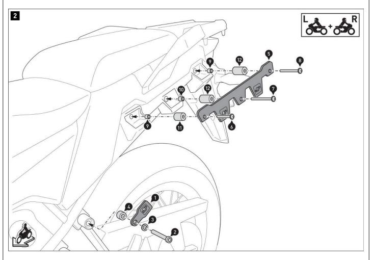
Screw the mounting brackets (1) onto both sides of the passenger footrest  $% \left( 1\right) =\left( 1\right) \left( 1\right)$ mounts.
