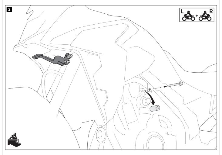
Remove the screws and bushings from the rear mounting point on both sides.
