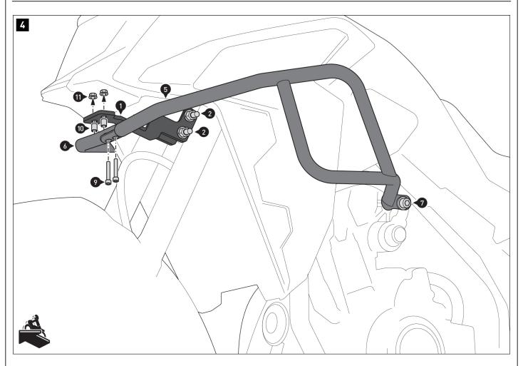
Screw the two upper crash bars (5) and (6) to the mounting bracket (1).
