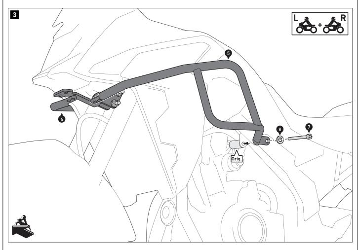
Screw the upper crash bars (5) and (6) to the vehicle on both sides using the original spacers (orig.).
