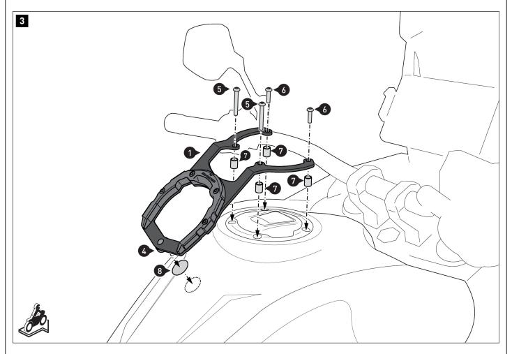
Carefully clean the surface of the tank so it's free of dirt and grease residue. Determine the support point of the vibration dampener (4). Then stick the adhesive protective foil (8) onto the support point.
