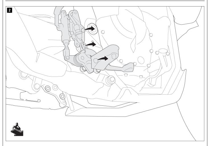
Unscrew the three marked screws from the footrest.
