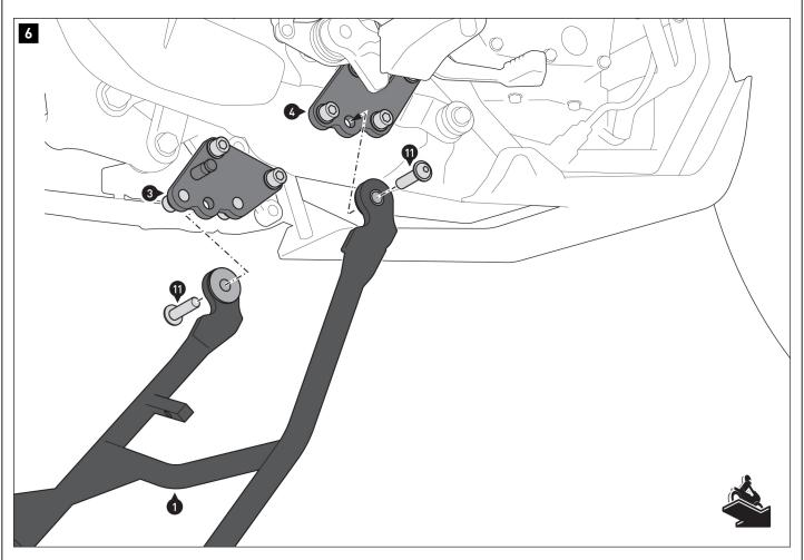
Screw the dismantled parts outlined in  $steps\ [1]$  and [2] back onto the vehicle; be sure to follow all manufacturer specifications.
