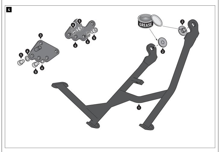
Coat the outside of the bearing bushings (2) with grease. Then insert the bearing bushings (2) into the openings on the centerstand (1).
