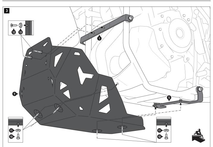
Screw the engine guard (9) to the mounting brackets (1) and (5). **A** WARNING: Use a liquid threadlocker!
